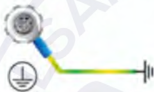
Figure 1: Socket-outlet protective earthing connection
