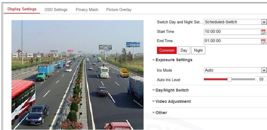
Figure 9-5 Day/Night Scheduled-Switch Configuration Interface
