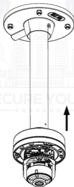
Figure 26, Install the Cap
