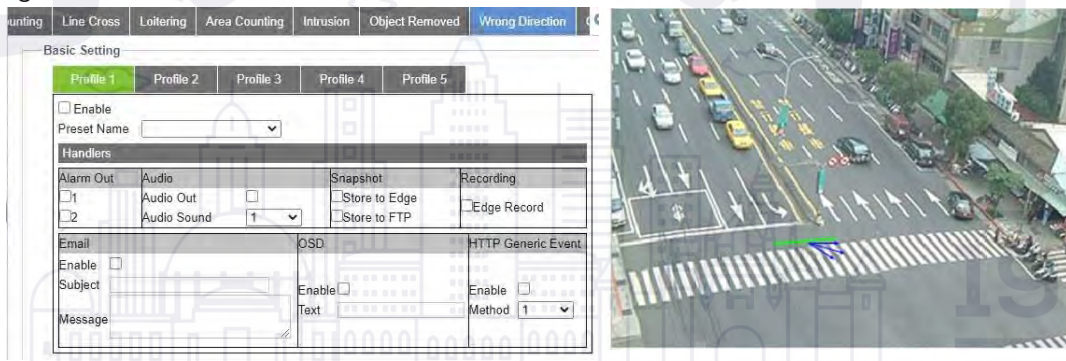
Figure: Wrong Direction Settings
