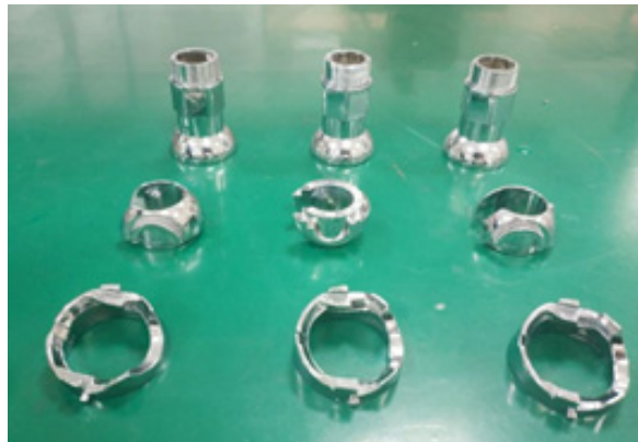
Figure 3.6 Samples after NEMA-4X salt spray test
