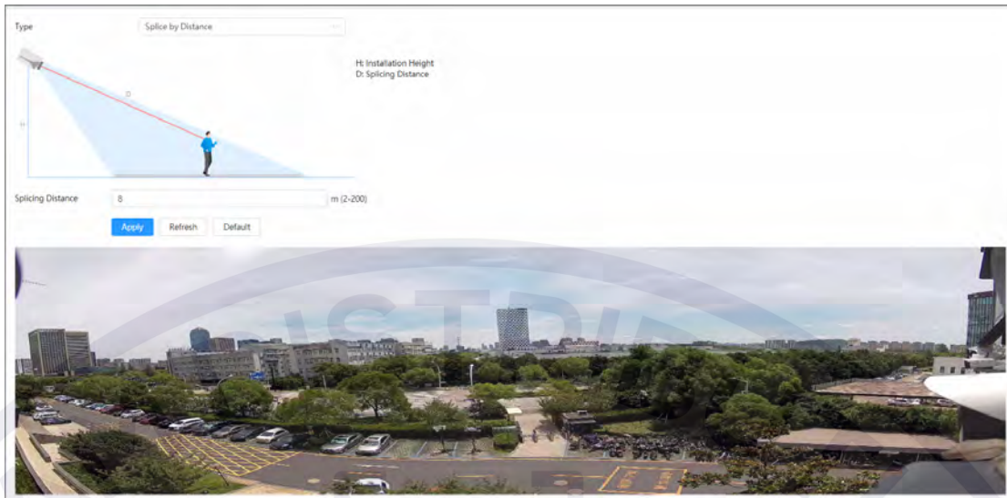
Figure 6-34 Splice by distance
