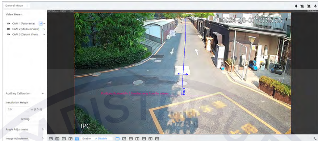
Figure 7-7 Configure auxiliary calibration
