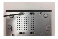
4. Turn the Device upside down and then fasten the screws.
