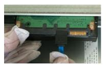
Connect one end of HDD cable to the HDD.
