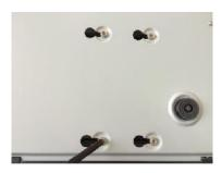
4. Turn the device to see the back side of it. Align the screws of the HDD with the holes on the back of the device, and then fix the screws.
