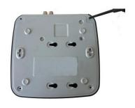
1. Remove the screws to take 2. Fix the screws on the HDD off the cover.
