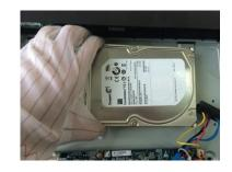
Place the HDD onto the Device.
