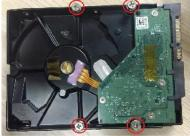
Fix the screws onto the HDD, but do not be fastened.
