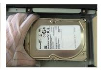
3. Put the HDD into the Device.
